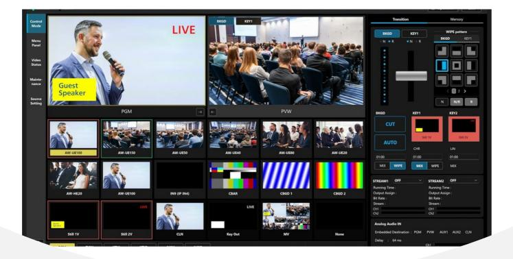
The Software Control Panel enables a networked PC\*or tablet\* connected to the AV-HSW10 main unit to be used for diverse operations and configurations.
