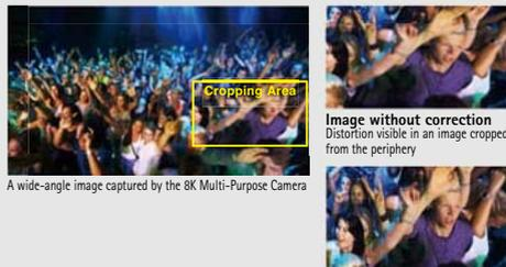
▲ Sample images after automatic wide-angle distortion correction
